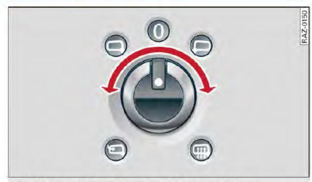
Fig. 40 Driver's door: knob for the exterior mirrors
