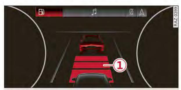
Fig. 112 Instrument cluster: request for driver intervention
