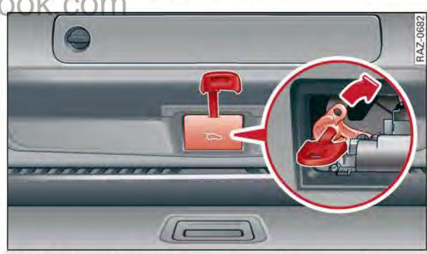
Fig. 31 Inner luggage compartment lid: access to the emergency release
