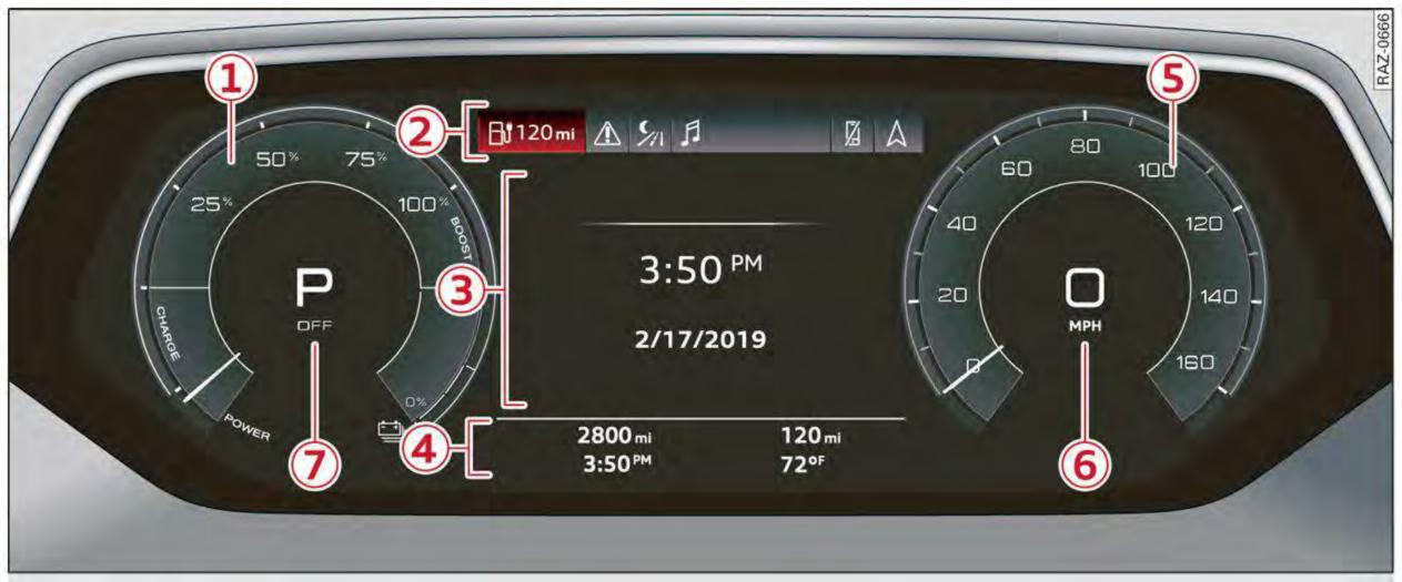
Fig. 2 Instrument cluster overview (Audi virtual cockpit)
