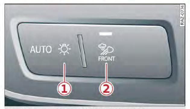
Fig. 35 Instrument panel: light button module
