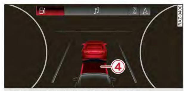
Applies to: vehicles with adaptive cruise assist: Fig. 114 Instrument cluster: distance warning
