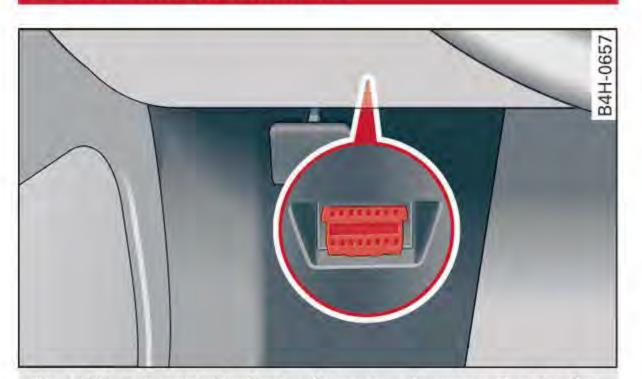
Fig. 180 Driver's side footwell: connection port for the On Board Diagnostic System (OBD)
