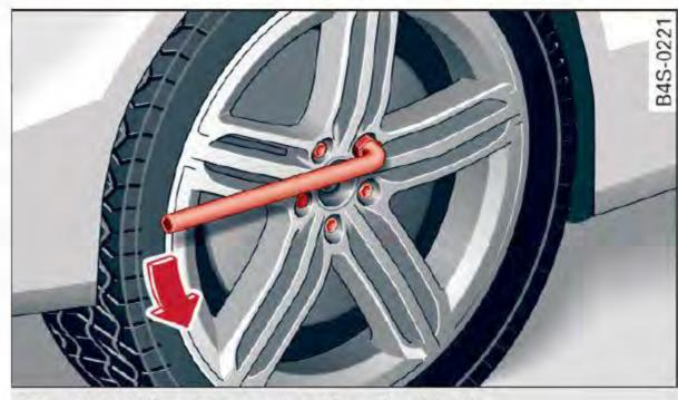
Fig. 167 Wheel: loosening the wheel bolts
