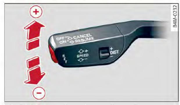
Fig. 106 Operating lever: changing the speed
