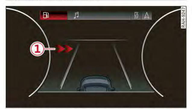
Fig. 121 Instrument cluster: directional display from the intersection assistant
