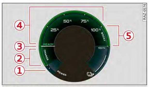
Fig. 6 Instrument cluster: power meter
