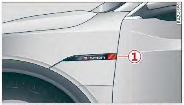
Fig. 85 Left front side of the vehicle: opening the highvoltage charging port door
