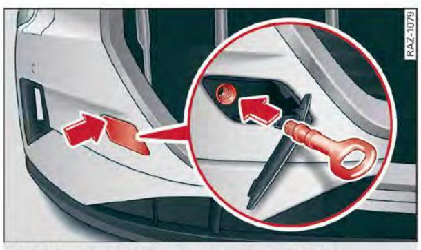
Fig. 172 Front bumper: installing the towing loop
