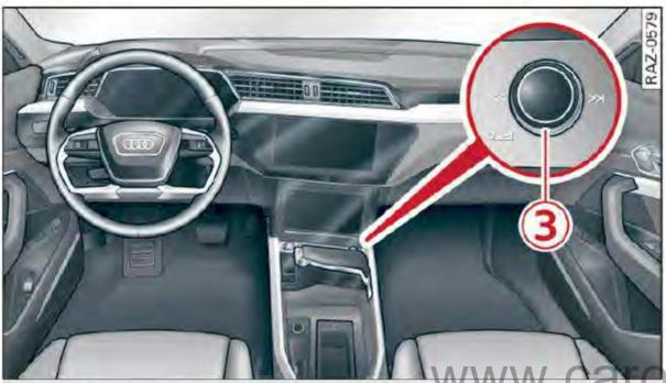
Fig. 20 Center console: MMI On/Off knob with joystick function
