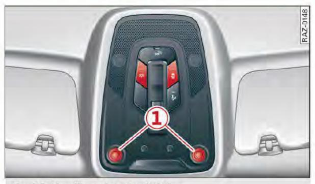
Fig. 38 Headliner: interior lighting
