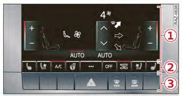
Fig. 79 Center console: lower display and switch panel
