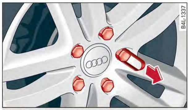
Fig. 165 Wheel: wheel bolts with caps
