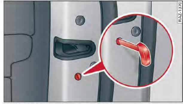
Fig. 23 Door: mechanically locking
