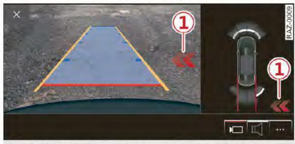
Fig. 130 Upper display: rear cross-traffic assist display
