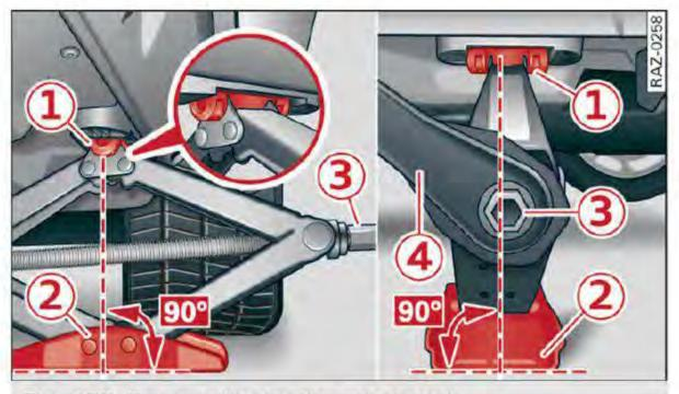
Fig. 169 Sill: positioning the vehicle jack
