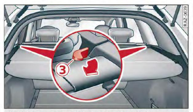
Fig. 70 Luggage compartment: removing the luggage compartment cover
