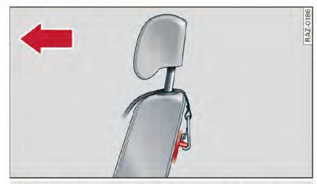
Fig. 64 Rear backrest: securing the upper belt to the top
