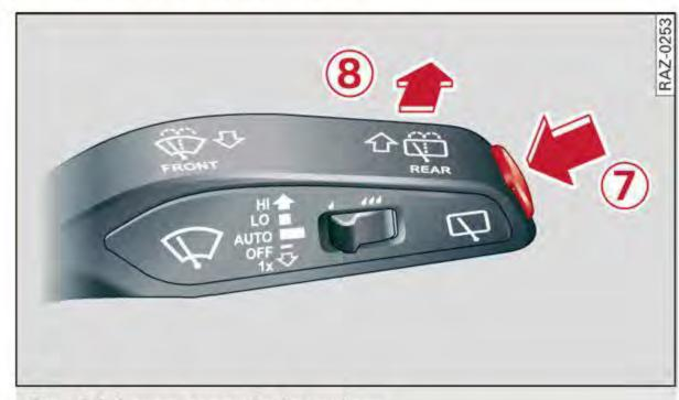
Fig. 44 Lever: rear window wiper
