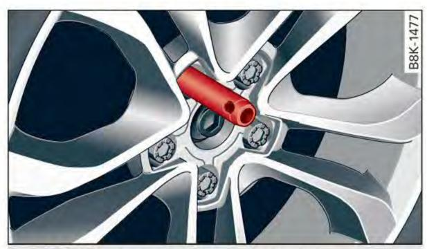
Fig. 171 Wheel: alignment pin in the top hole
