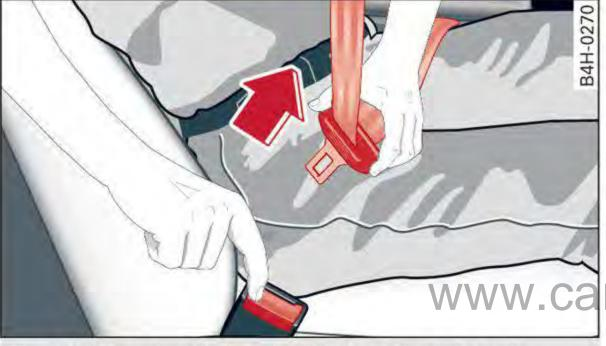
Fig. 58 Releasing the belt buckle from the belt latch
