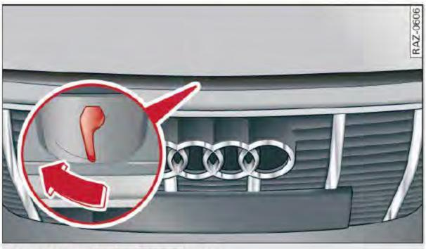
Fig. 152 Unlocked hood: lever
