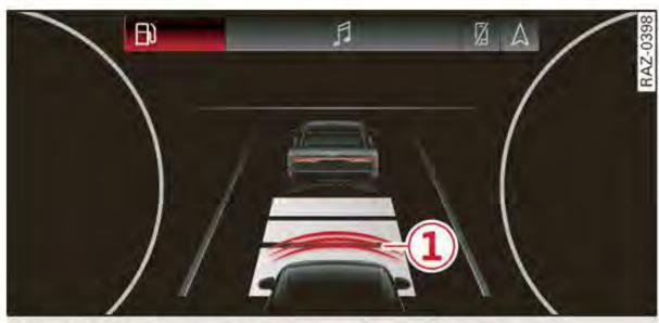
Fig. 111 Instrument cluster: safe start monitor
