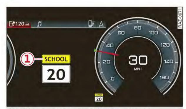
Fig. 98 Instrument cluster: traffic sign recognition
