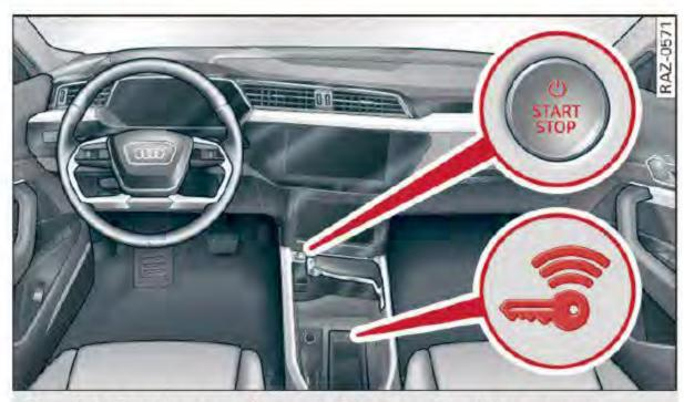
Fig. 81 Center console: switching on the drive system
