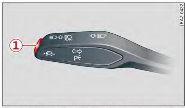
Fig. 107 Turn signal lever: button for lane guidance and lane departure warning WWW.Caro
