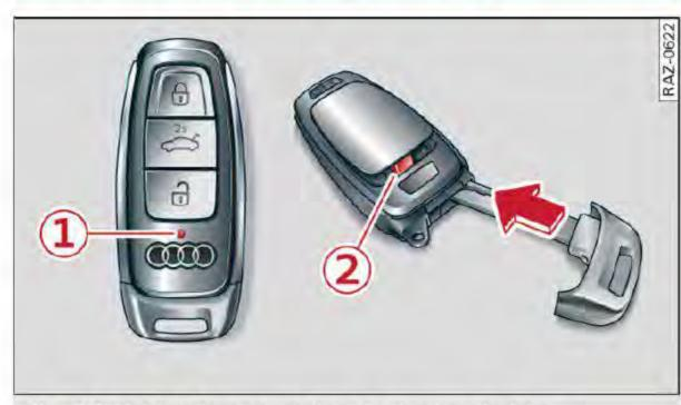
Fig. 26 Vehicle key: removing the battery holder
